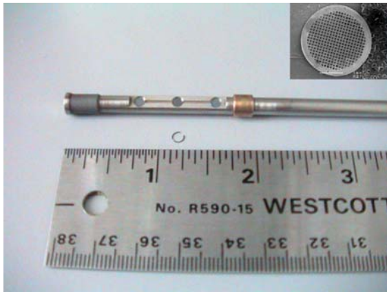
Fig. 2 One of the thermophoretic samplers used in this study. Inset: a low magnification micrograph of one of the sample grids used in this study
